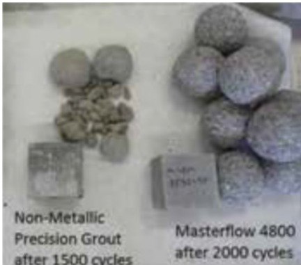
Figure 3. Grout samples after 1500 and 2000 cycles.
